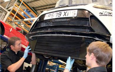
Pro Alloy intercooler slots neatly into place. It's built to very high standards and is a fair bit larger than the original RS item as you can see
