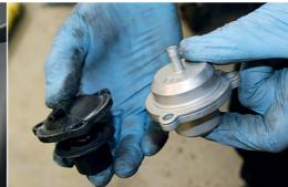
Mountune inlet, air box and recirculating valve are all part of the MR375 kit
