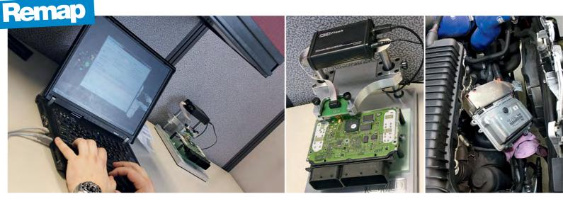
The RS ECU is removed and flashed with Mountune's 'Ford Approved' MR375 engine map
