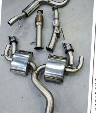
Made from aircraftgrade stainless steel and featuring smooth radius mandrel bends and TIG-welded joints, Milltek exhaust is top notch
