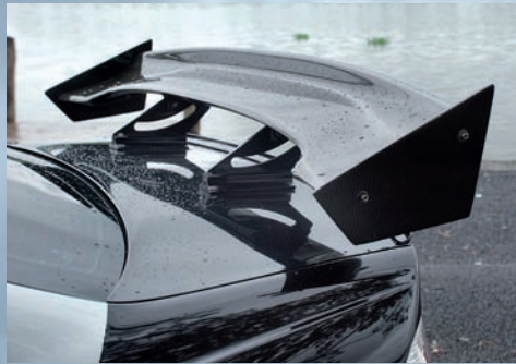
Massive rear-wing must add some amount of drag.
